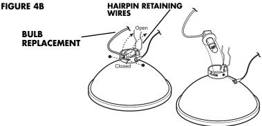
REPLACING THE AREA LIGHT BULB:
